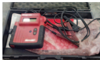
>> Top Left: IF YOU ARE HAVING ISSUES with a unit not starting this battery/starter tester will quickly identify or eliminate some issues.
