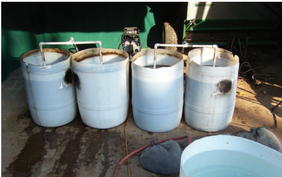
➤ THIS IS OUR BREWING SET-UP with the air compressor in the middle of the four containers and PVC piping branching off of that.
