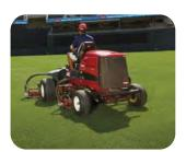
diesel engine, this unit offers a nimble and maneuverable design for mowing in a wide range of conditions. The Reelmaster 5210 is lightweight and productive with a 100inch width of cut. It is available in standard 2 wheel drive or add on the CrossTrax all-wheel drive system.
