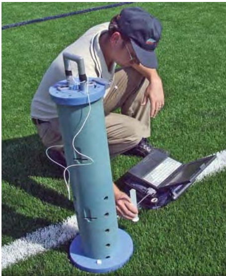
» Turf Diagnostics technician measuring field temperature and infill depth as part of a field evaluation.
