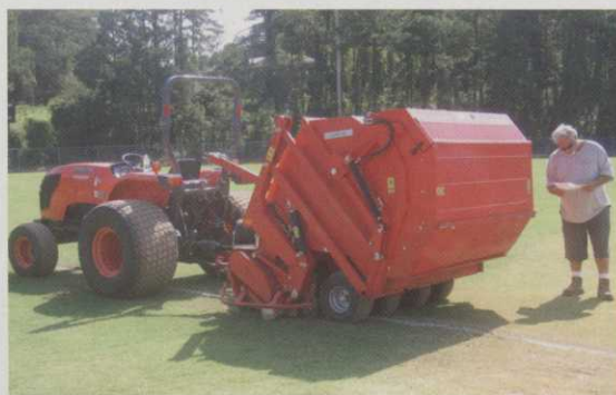
» Above: IF CORE CULTIVATION DEPTH penetrates the topdressing layer, or sand-cap (top photo), these cores should be removed to prevent drainage from being compromised by the native soil that is brought to the surface.
