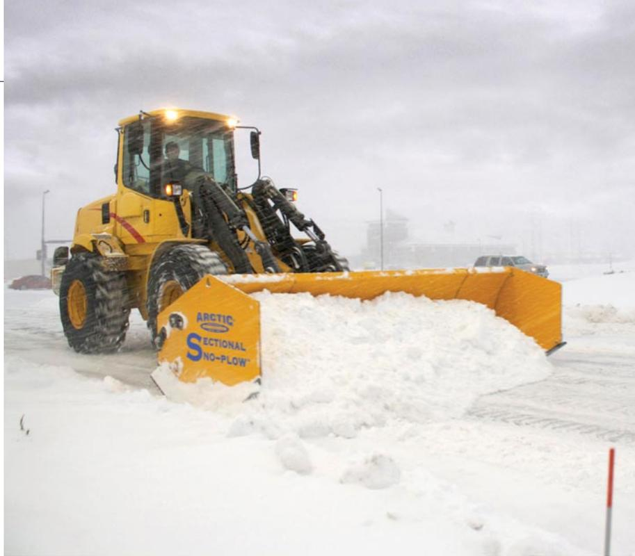
» USING A PLOW that incorporates features designed for fast, efficient removal of snow and ice will reduce the need to use salt, which is less effective in cloudy, colder conditions. Photo courtesy of Randy Strait.
