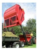
verti-cutting, flail mowing, core collection and debris clean up applications into one machine. The Turf Tidy's fully floating cutting head follows the ground's contours, ensuring accurate cutting and pick-up. The unique turbo fan makes a clean sweep of leaves, pine needles, paper, aeration cores and grass clippings. The
