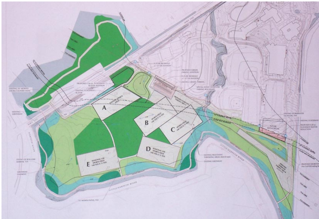
➤ A MAP OF THE ENSWORTH SCHOOLS PROPERTY defining property lines, rivers, the stream, the highway, buildings, parking lots, athletic fields, greenway, cross country course, the flood plain, floodway, floodway buffer, pond, tennis courts, the storm water outflows and all the management zones.
