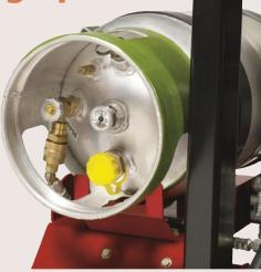
>> PROPANE-FUELED COMMERCIAL MOWER CYLINDER EXCHANGE PROGRAMS usually include installation of a cage and replacement of empty cylinders during regularly scheduled deliveries. The cylinders can be refueled via a centralized, on-site refueling infrastructure.
