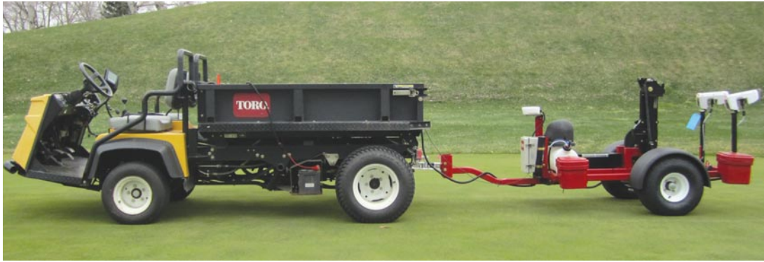
>> Figure 1. MOBILE SPATIAL MAPPING devices for sports fields. Top: multiple sensor device to map soil moisture, salinity, penetrometer resistance, turf quality, and topographic relief. Bottom: accelerometer device that is similar to the Clegg Accelerometer to determine surface hardness (images courtesy of The Toro Co.).
