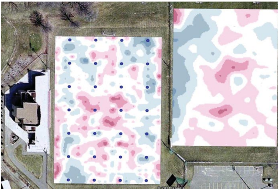
>> Figure 2. SOIL HARDNESS determined by the Toro accelerometer presented in standard deviation format maps that illustrate the lowest and highest hardness areas in a field. These can often be related to soil moisture and traffic patterns. Blue dots are irrigation heads.
