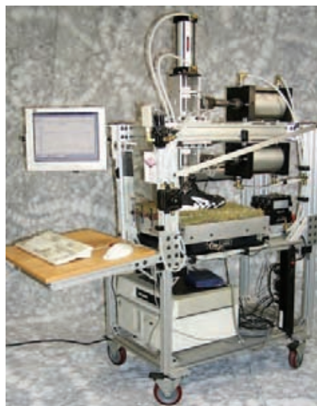
» THIS PNEUMATIC FOOT can simulate athlete maneuvers like starting, stopping and cutting, and Ohio State researchers can test small samples in the lab rather than having to install costly plots.
