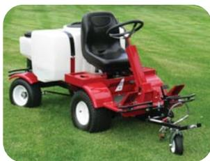
also features a hydrostatic drive with 25' hose for stencil work.
