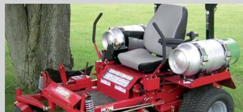
**>> PROPANE CYLINDERS** are typically installed horizontally on a mower, and are either located in the mower's rear, or on the sides, as shown here.
