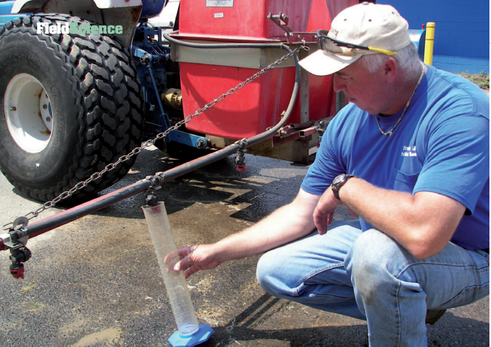
➤ A graduated cylinder (ml) was used to check each nozzle for a calculated spray volume equivalent to 0.4 GPM (i.e. 380 ml in 15 seconds).
