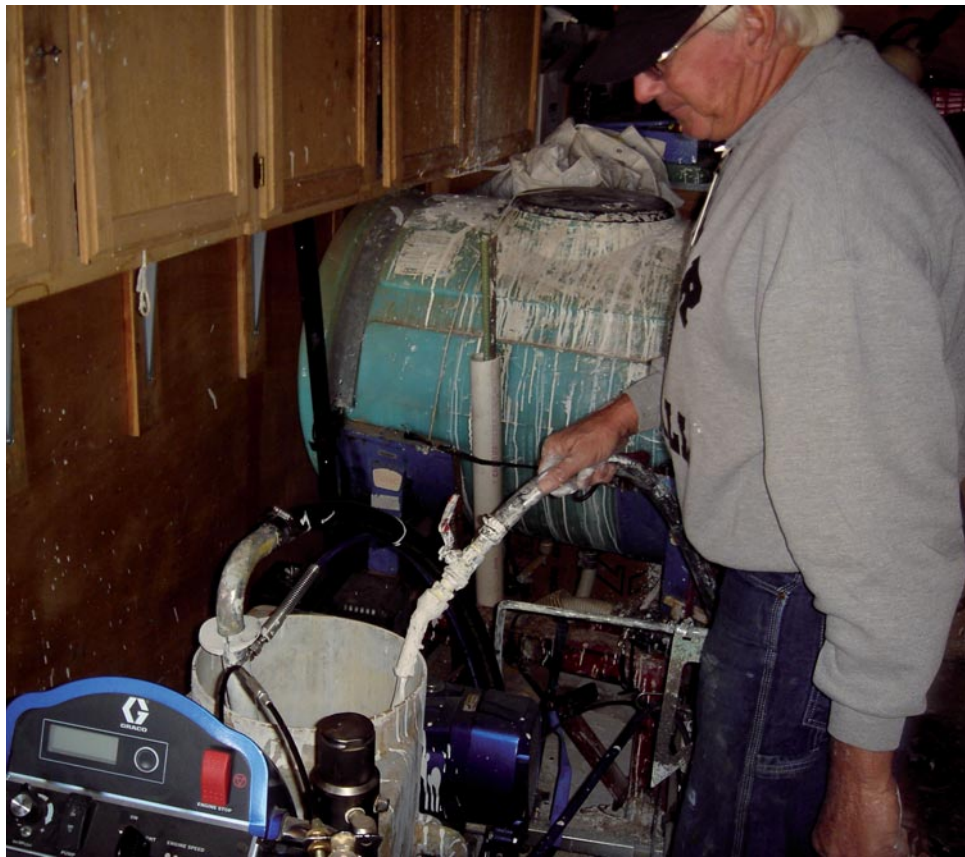
» Jim Wilson loads a striper with diluted turf paint.
