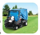
grass, and a verticut option that performs two jobs in one pass. The hopper lifts to a height of 6 ft. to dump directly into a cart or waste dumpster, avoiding the need to handle material twice. **www.deweze.com**
