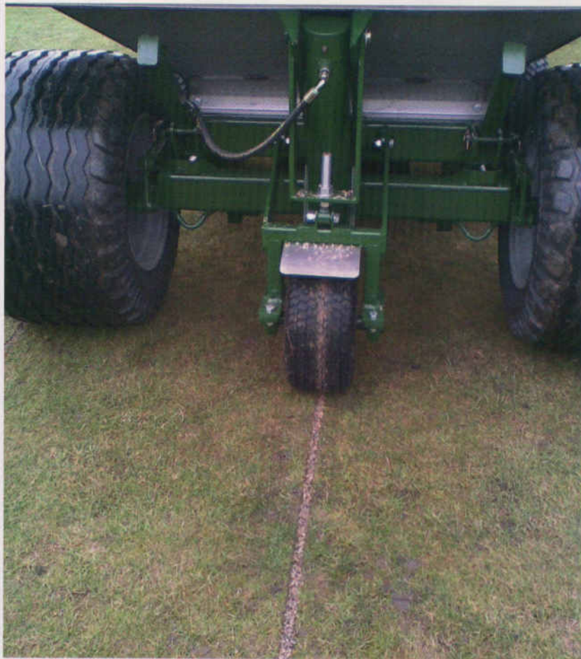
Three-ton Gravel Band Drainer installing gravel to surface. Aggregate can also be set down in the trench.
