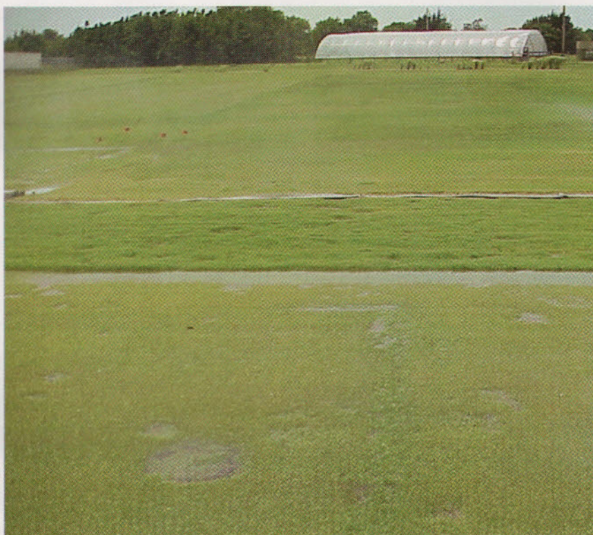
Figure 2. Runoff slows and puddles as it flows across turf mowed at 0.5 inches and encounters a buffer mowed at 2.0 inches on a 5% slope.
