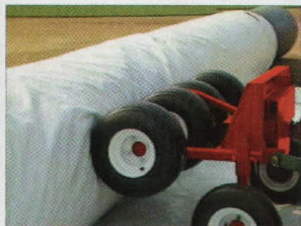
A portable rolling device for covers marketed by Covermaster.
