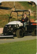
**Bobcat's** new 2300 4x4 utility vehicle can mow, sweep, and move materials with its **RapidLink** attachment system, which can lift loads up to 500 lbs. as high as 2 ft. The 20-hp unit has the exclusive **IntelliTrak** drive system. Cab provides legroom, storage spaces, cup holders, and a 12-volt power adapter on the dash panel.
