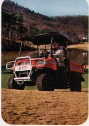
The **RTV900** is a durable UV from **Kubota** that features a 3-range variable hydro transmission, more traction in reverse speed, wet-disc brakes, a hydraulic bed-lift system, and an improved tailgate design.
