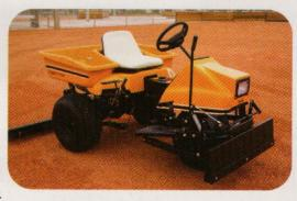
Standard features include engine kill switch, headlight, 12-volt power source, cup holder, and exclusive wrap-around rear-hinged cargo box. Mid- and rear-hydraulic lifts accommodate a variety of attachments.
