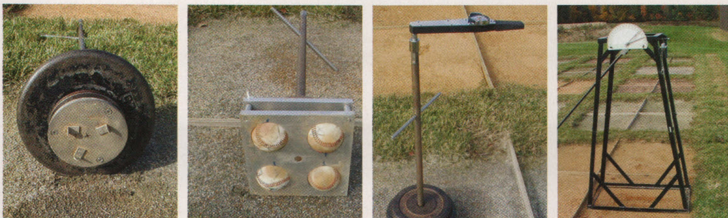
Devices used for measuring traction, static ball-to-surface friction, and dynamic ball-to-surface friction of skinned infield plots at the University of Connecticut.
