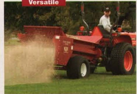
Both Turf Tiger Cub models can spread wet or dry, coarse or fine materials.
