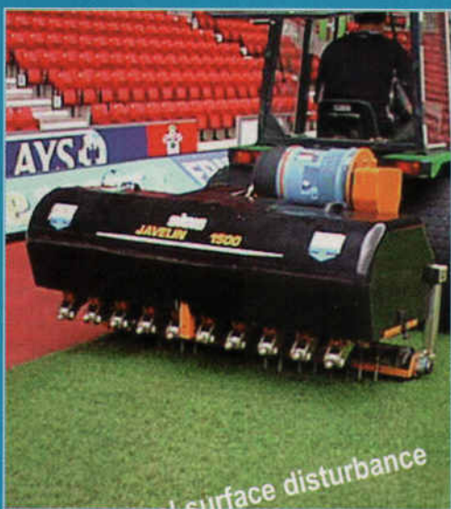
Clean air is blasted into the root zone at a rate of 3cu.ft. per minute
