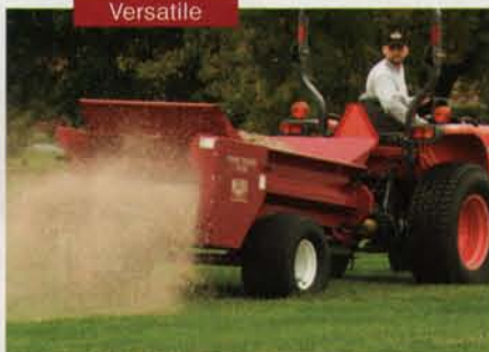
Both Turf Tiger Cub models can spread wet or dry, coarse or fine materials.
