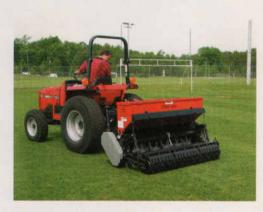
Patented vibrating tines extensively fracture soil without destroying existing turf. Machine has swing hitch that allows you to turn around objects without tearing turf. Available with either ground driven or electric drive seed hopper. First Products/800-363-8780 For information, circle 101 or see http://www.oners.ims.ca/4569-101
