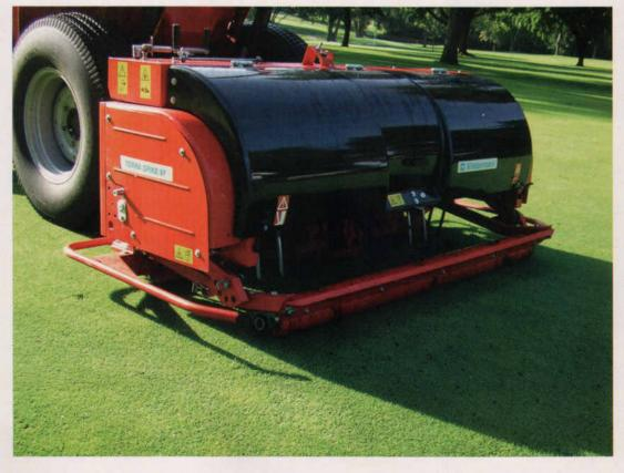
So when using SUD aerifiers, whether going deep or shallow, you should avoid using solid tines and stick to coring tines for compaction relief. Solid tines can effectively be used with deep tine "heaving-type" aerifiers with little or no damage to the turf. With solid tines ranging from 3/16 to 1 inch in diameter and 6 to 16 inches in length, the ground doesn't need to be bone dry but only needs sufficient moisture for optimal penetration and compaction relief.
