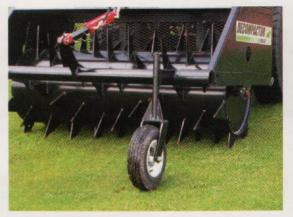
than the recommended 1-2 mph for most mechanical driven deep tine aerators. The machine fractures the soil between visible holes to allow faster infiltration of air, water, and nutrients into the soil. This non-localized approach to decompaction allows the SMARTURF to cover more ground in less time, which can conserve resources.
