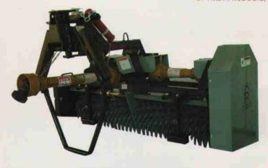
THE VC-60 IS DESIGNED FOR CONTINUOUS HEAVY DUTY OPERATION ON ALL TYPES OF SPORTS TURE. THE UNIT HAS A PATENTED SWING HITCH THAT ALLOWS THE OPERATOR TO VERTI-CUT AROUND OBJECTS WHILE TURNING, WITHOUT TEARING THE ESTABLISHED TURE. PIVOT POINTS DESIGNED ON THE HITCH ALLOW THE UNIT TO FLOAT OVER UNEVEN TERRAIN. THE VC-60 CUTTING DEPTH IS EASILY ADJUSTED IN THE FIELD, WITHOUT TOOLS "UP TO 1% INCHES DEEP" USING QUICK RELEASE PINS.
