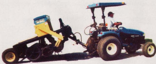
**Seeding is Believing** – The Quick Slit Seeder follows the ground contours accurately and plants seeds at a constant depth in its own prepared mini seedbed. This unit is also a cultural tool in that it acts as a grass root pruner by cutting or breaking the grass plant roots. For the survival of the grass plant, it must immediately put all of its resources into growing new roots, resulting in stronger plants with better root structures.
