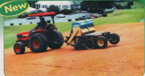
**Seeding is Believing** – The Quick Slit Seeder follows the ground contours accurately and plants seeds at a constant depth in its own prepared mini seedbed. This unit is also a cultural tool in that it acts as a grass root pruner by cutting or breaking the grass plant roots. For the survival of the grass plant, it must immediately put all of its resources into growing new roots, resulting in stronger plants with better root structures.
