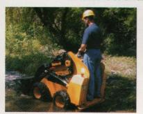
separate attachments. Machine is made to save labor on jobs such as small-scale dirt handling, utility installation, and lifting projects. Units have oil coolers and easy access to battery.
