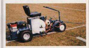
The Jaydee Drive Liner is a self-propelled riding line marker. The 35-gallon paint tank carries enough marking material for a complete game field, or several practice fields. The 2-gallon flush tank cleans the discharge lines for work breaks, travel, or overnight. The center or side-mark spray shields are always operator-visible. A nearly zero turning radius reduces or eliminates back and turn maneuvers.
