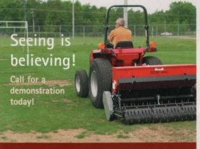
THE SE-60 SEEDA-VATOR IS THE ONLY SEEDER ON THE MARKET TODAY WITH THE FLEXIBILITY OF PRIMARY SEEDING OR OVERSEEDING WITH THE SAME MACHINE. THE UNIT HAS A PATENTED SWIVEL HITCH THAT ALLOWS THE OPERATOR TO TURN AROUND OBJECTS WITHOUT TEARING ESTABLISHED TURF. THE CLEATED ROLLER CAN BE PINNED TO GAGE TINE DEPTH. THE SE-60 USES PATENTED VIBRATING TINES TO FRACTURE THE SOIL, RESULTING IN AN IDEAL SEEDBED. THE SEEDA-VATOR COMES WITH EITHER GROUND DRIVEN OR ELECTRIC DRIVE SEED HOPPER.
