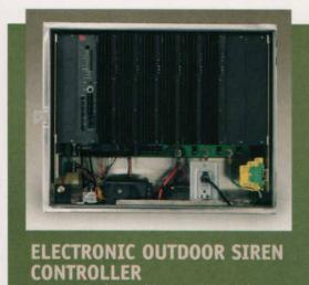
Federal Signal has introduced the UltraVoice, a controller for outdoor electronic sirens. It is meant to provide control of high-powered sirens as well as indoor speaker systems. The controller produces amplified audio signals including seven built-in warning tones, live public address, and up to 16 variable length pre-recorded voice messages
