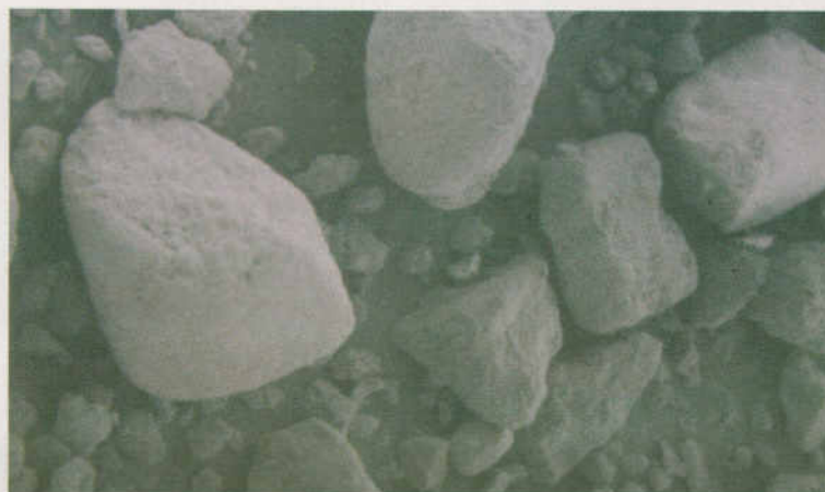
You can see the sharp edges and angles of the sand particle (below) compared to the smooth edges of the rubber particle.
