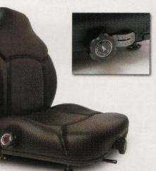
sion seat with hydraulic shock and automotive-type spring seating system. Adjustable lumbar support, adjustable back angle and 6-in. travel fore & aft adjustment. Prime Line/217-324-9400 For information, circle 183
