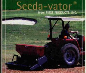
THE SE-60 SEEDA-VATOR IS THE ONLY SEEDER ON THE MARKET TODAY WITH THE FLEXIBILITY OF PRIMARY SEED-ING OR OVERSEEDING WITH THE SAME MACHINE. THE UNIT HAS A PATENTED SWIVEL HITCH THAT ALLOWS THE OPERA-TOR TO TURN AROUND OBJECTS WITHOUT TEARING ESTAB-LISHED TURF. THE CLEATED ROLLER CAN BE PINNED TO GAGE TINE DEPTH. THE SE-60 USES PATENTED VIBRATING TINES TO FRACTURE THE SOIL, RESULTING IN AN IDEAL SEEDBED. THE SEEDA-VATOR COMES WITH EITHER GROUND DRIVEN OR ELECTRIC DRIVE SEED HOPPER.
