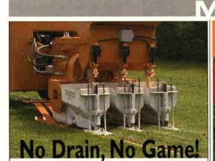
WaterWick's patented gravel-vein injection system creates a permanent answer to chronic wet turf problems. So the game goes on without delay.
