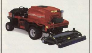
The Cushman® Envirojet™ pull-behind chemical injection system applies amendments directly to the turf root zone. The patented system cleanly and safely saturates the target area to apply fertilizer, treat fungal infestations or other applications. For the name of your local Cushman® Envirojet™ dealer, or a FREE demonstration, just call 1-888-922-TURF (8873).
