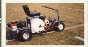
The Jaydee Drive Liner is a self-propelled riding line marker. The 35-gallon paint tank carries enough marking material for a complete game field, or several practice fields. The 2-gallon flush tank cleans the discharge lines for work breaks, travel, or overnight. The center or side-mark spray shields are always operator-visible. A nearly zero turning radius reduces or eliminates back and turn maneuvers.
