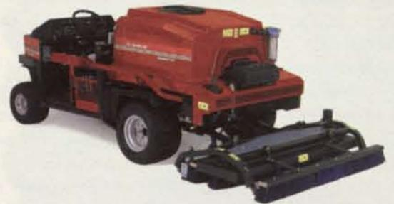
The Cushman® Envirojet™ pull-behind chemical injection system applies amendments directly to the turf root zone. The patented system cleanly and safely saturates the target area to apply fertilizer, treat fungal infestations or other applications. For the name of your local Cushman® Envirojet™ dealer, or a FREE demonstration, just call 1-888-922-TURF (8873).
