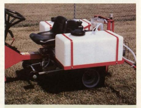
The grounds maintenance staff at Lewis Palmer High School, Monument, CO extensively uses the spray boom for their herbicide applications with great results, reports Tru Mark. The optional spray boom on their RS-500 Rider can function as a field marker (end zone marking), herbicide sprayer, and fertilizer applicator for large sport fields.
