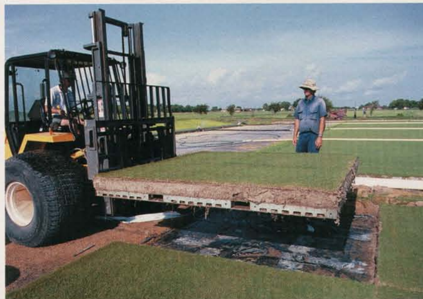
A forklift moves an 8 x 8-ft. module of turf, grown at the Turfgrass America farm in Bay City, TX.
