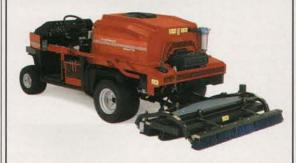
The Cushman® Envirojet™ pull-behind chemical injection system applies amendments directly to the turf root zone. The patented system cleanly and safely saturates the target area to apply fertilizer, treat fungal infestations or other applications. For the name of your local Cushman® Envirojet™ dealer, or a FREE demonstration, just call 1-888-922-TURF (8873).
