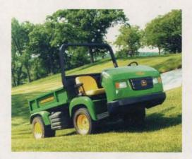
Available in 23.5-hp diesel and 26-hp gas versions, the vehicles have a 5-speed, fully synchronized transmission that let's you keep going without stopping to change gears. Hydrostatic steering provides for precision controls and a tight turning radius. With a 2,650-lb. payload capacity and a hydraulic lift, the ProGator can handle heavy loads.
