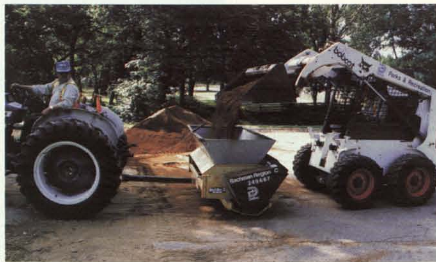
Top-dressing infields can be done fairly quickly and easy with bulk infield conditioners, saving time and money.
