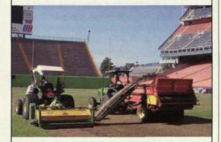
Strip and remove a layer of turf from a half-inch to 2 inches deep, making the resodding of tees, greens, fairways and sports fields quicker and more efficient. The Field TopMaker is available in two models.
