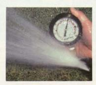
It's important that conditions for good irrigation system performance are in place, including proper pressure, head spacing and nozzle selection, and appropriate sprinkler alignment.
