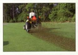
1. Commercial quality fine turf verti-cut 2. PTO powered - 20 to 30 H.P.
