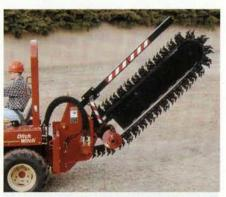
attachment replaces the H412 and features a sealed Eaton motor and new bearings and headshaft to eliminate need to pre-load bearings. The larger lifting cylinder offers more capacity and effectiveness, especially when coupled with the optional 5-foot boom, says the company. This model also uses components common to Ditch Witch H313 and H314 attachments to offer increased parts supply. For more information, circle 139
