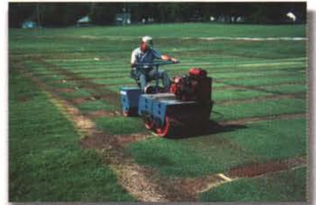
The turfgrass traffic simulator has drums with cleats attached, to simulate one football game under wet conditions.
