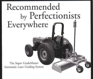
At LaserLeveling, we realize the importance of perfection, this is why we design box scrapers specifically for the sports turf industry. The Super GradeMaster allows you to push and pull material, giving you more flexibility and control than ever before. If you're looking to take your grading to a new level, look to Laser Leveling.
